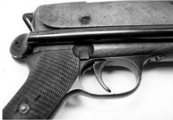
Right side view of the trigger area. Fire selector button is shown just above trigger.
